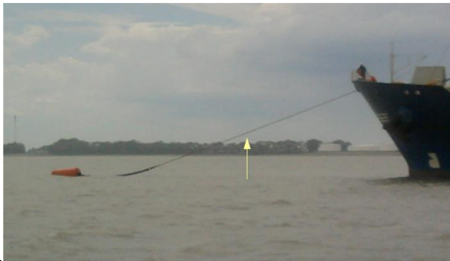
The ship continues to advance and begins to embark the chain and buoy system.
